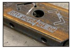
■ Clear Marking/Etching allows all assembly instructions, part numbers, weld lines and more to be automatically applied to all four sides. This adds value to the process by reducing measuring and errors during fabrication.
