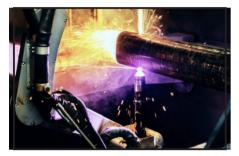
■ 360° processing. The specialised robotic arm enables the Metaltek XB to cut and mark underneath. This gives the ability to cut rectangular hollow section on all four sides with full 45 degree bevels from any direction on any face.
