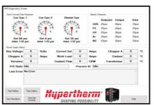
■ Diagnostics screens give readouts on internal information. Displays gas selections, inlet pressures, flow settings, temperature and coolant flow.
