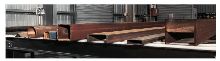
■ Automated material handling. The material handling system combines both cross-feed chain conveyors and servo driven position controlled roller conveyors. Material is loaded onto the in-feed system by the operator where it is fully processed and rolled out of the out-feed system automatically. All conveyor functions are controlled by the CNC controller. Manual override is available for operator control of conveyors
